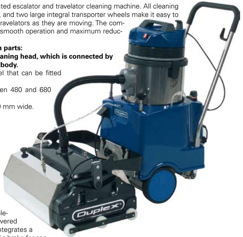
**a) The machine body** is built completely from stainless steel and is covered by a robust polypropylene chest. It integrates a powerful vacuum, detergent tank and a brake for controlling the machine on the escalator or travelator.
